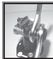
Raccordement entrée rob type E
