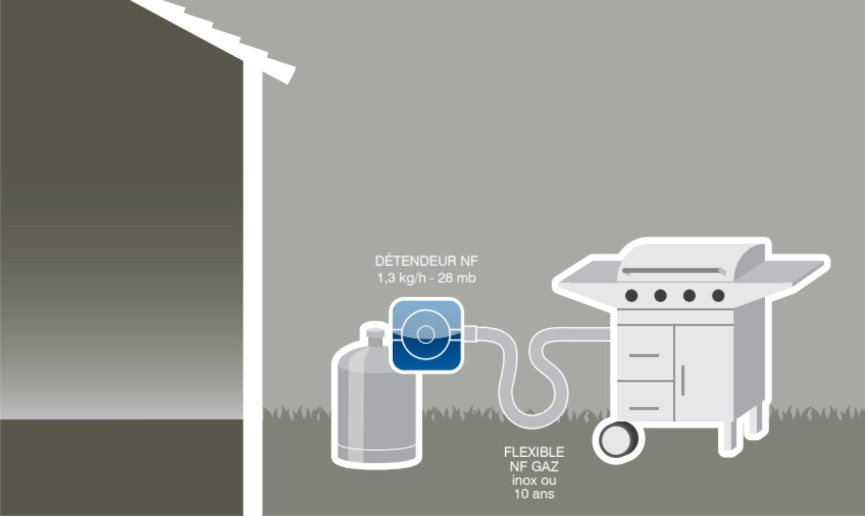
A diagram showing a gas connection system. On the left, a grey gas cylinder is connected to a blue square pressure-reducing valve. A white flexible gas hose runs from the valve to a stainless steel grill on the right. The grill has four burners and a lid. The background is a dark grey gradient with a white outline of a house on the left and a grassy area at the bottom.
